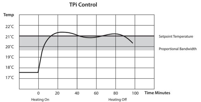
*Example – Program 1 on the thermostat is 21°C for 06:30am and the room temperature is 18°C. The thermostat will start the heating at 06:30am and the heat will start to increase then but will switch itself off before it reaches temperature and allow the room temperature to increase naturally – this cycle may begin again if the thermostat isn't reaching temperature.*
