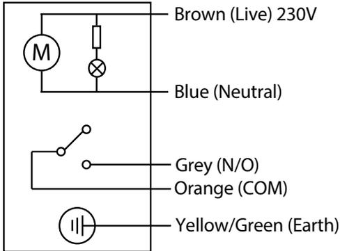
The auxiliary switch can be used as an interlock facility, thereby ensuring any auxiliary equipment is switched OFF when the valve is in the closed position. When the valve is in the fully open position the auxiliary equipment will be switched ON.\*
