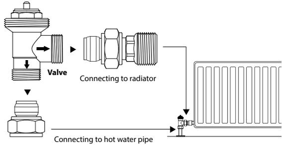
Figure 2.0 Valve Installation
