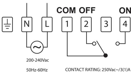
If mains voltage output is required, terminals L & 1 must be electrically linked. The cable link is provided with this timeswitch.
