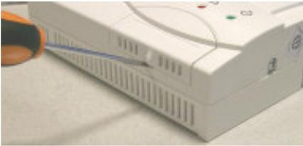
1\_ Turn off the detector, unplug it from the mains and use a screwdriver to lever off the little cover under the three LEDs (Fig. 12).
