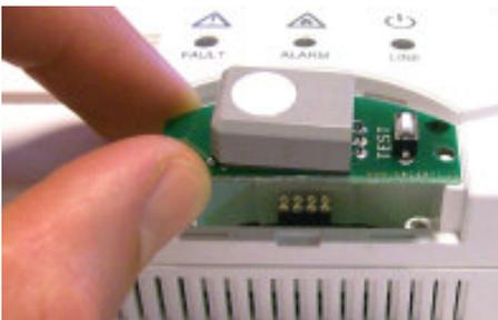
3\_ Remove the **Sensor module** to be replaced (Fig. 14).
