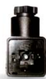
1578501 Quick connection connector DIN 43650, suitable for all IM2 coils. Cable gland Pg9 (cable diameter 6÷8 mm). Adjustable cable outlet in 4 positions every 90°.
