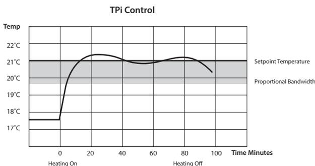
*Example – Program 1 on the thermostat is 21°C for 06:30am and the room temperature is 18°C. The thermostat will start the heating at 06:30am and the heat will start to increase then but will switch itself off before it reaches temperature and allow the room temperature to increase naturally – this cycle may begin again if the thermostat isn't reaching temperature.*
